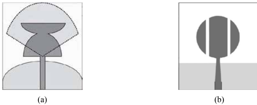
Fig. 15. Some other forms of parasitic patch band-notched UWB antennas [25, 26].
