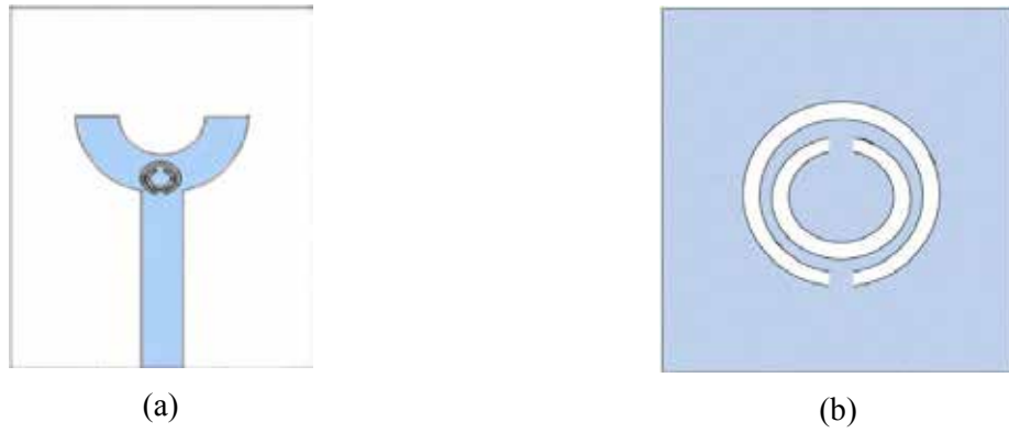
Fig. 10. (a) UWB antenna having embedded SRR in the patch; (b) SRR cell [18].
