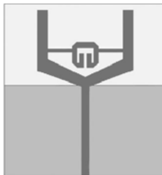
Fig. 12. UWB antenna with an open loop resonator attached to the center of its patch [20].
