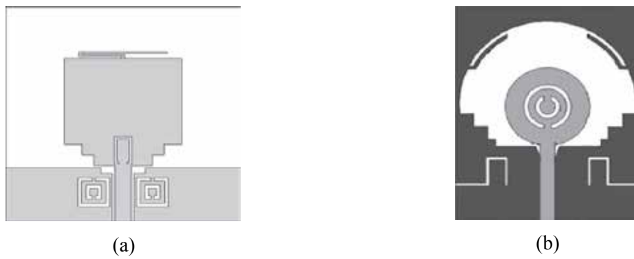
Fig. 18. UWB antennas incorporating multiple techniques to realize notched-band [20], [21].
