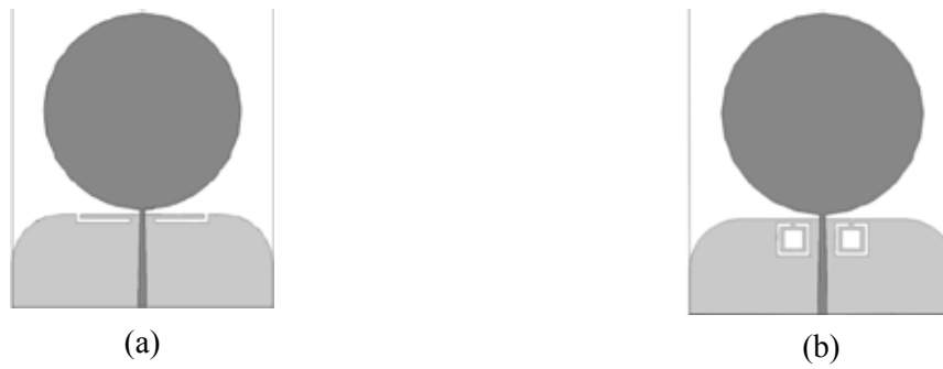
Fig. 5. Antennas with slot in ground plane: (a) Quarter wave; (b) Half wave [13].
