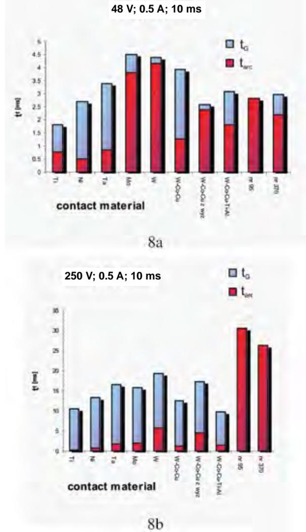
**Fig. 8.** Comparison of total discharge time ( $t_t$ ) and portion of the glow duration ( $t_g$ ) for tested contact materials when interrupt inductive load DC (0.5A, 10 ms) at different voltage value (48 V and 250 V) in air under normal pressure ( $\sim 100$  kPa).
