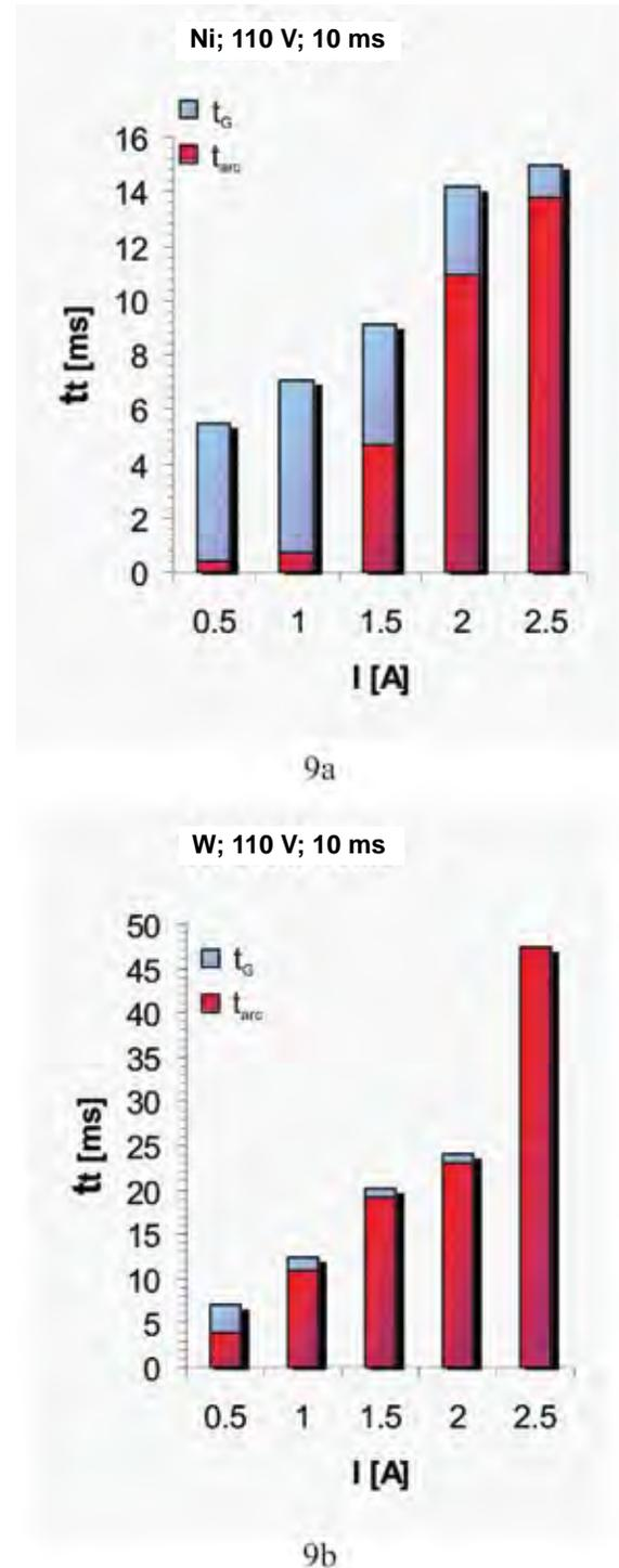
**Fig. 9.** Comparison of total discharge time ( $t_t$ ) and portion of the glow duration ( $t_g$ ) for nickel and tungsten as contact materials when interrupt inductive load DC (110 V, 10 ms) at different current value in air under normal pressure ( $\sim 100$  kPa).
