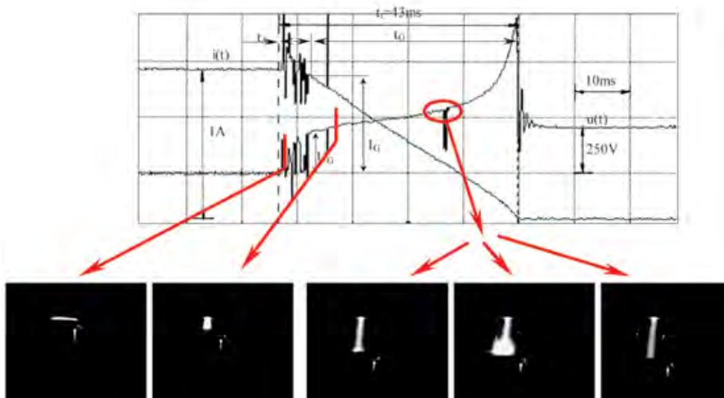
**Fig. 3.** The unstable arc to glow transition when use the nickel contacts (250 V, 1 A, 40 ms, air  $\sim 100$  kPa) ( $t_c$ ,  $t_{ARC}$ ,  $t_g$  – total, arcing and glow discharge time respectively,  $U_g$  – glow voltage,  $I_G$  – arc to glow transformation current value).
