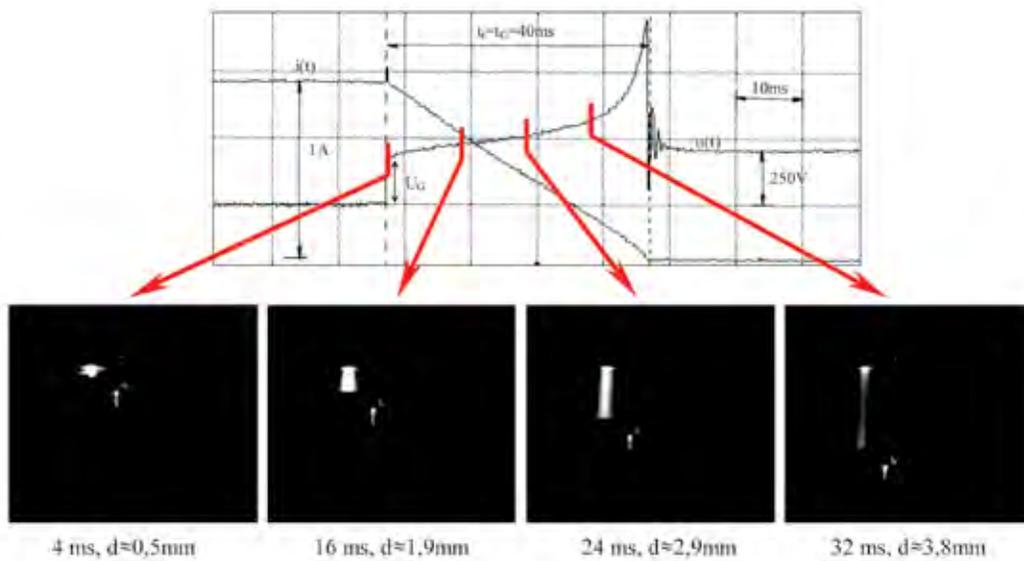
**Fig. 2.** Glow discharge triggered at the beginning of the contact separation when brake inductive load DC (250 V, 1 A, 40 ms) in air ( $\sim 100$  kPa) with contacts made of fine nickel. ( $t_c$ ,  $t_g$  – total and glowing time respectively,  $U_G$  – glow voltage).
