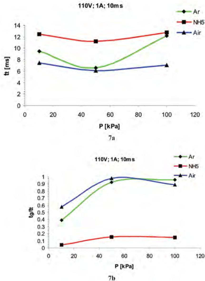
**Fig. 7.** Variation of the discharge time ( $t_t$ ) and the portion of the glow duration ( $t_g/t_t$ ) versus pressure (P) when interrupt inductive load DC (110 V, 1A, 10 ms) in selected gaseous mediums (air, argon, nitrogen-hydrogen 5% mixture) with contacts made of the fine nickel.
