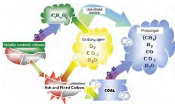
Fig. 2. Overview of coal gasification process.
