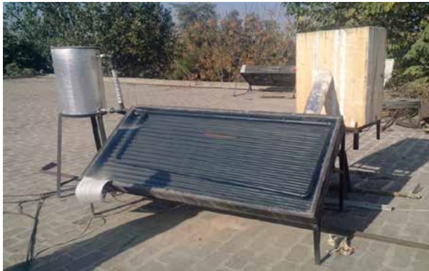
Fig. 1. Front view of the flat plate solar air heater used in the experiment.
