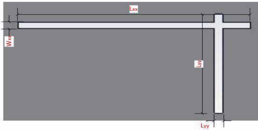
Fig. 5. L-shaped slot inserted in the patch for introducing band notch.
