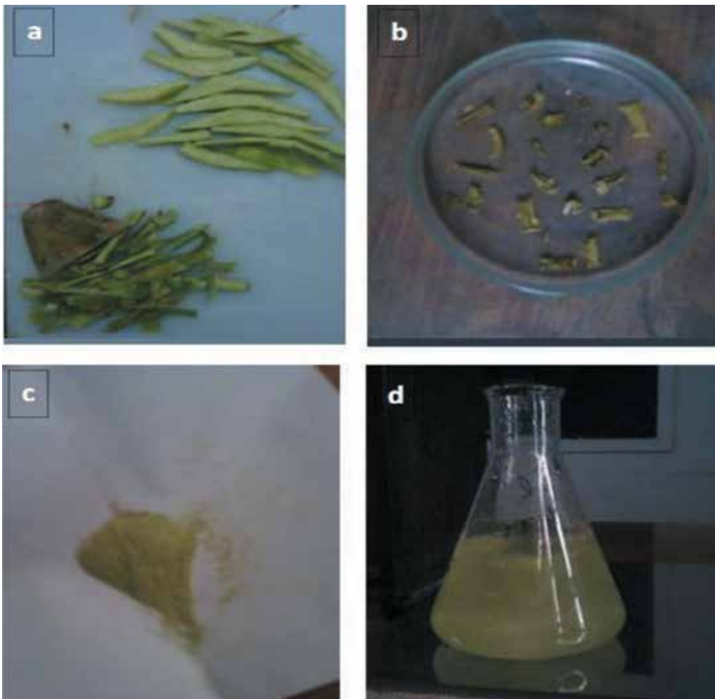
Fig. 2. Extraction and preparation of coagulant solution.
