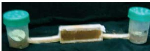
**Fig. 1.** Tunneling test apparatus.
