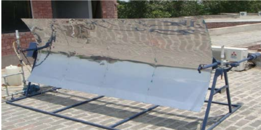
Fig. 6. Reflecting Surface of the experimental rig.
